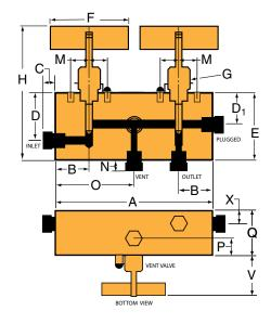
*G* - Packing gland mounting hole drill size H Dimension is with stem in closed position. All dimensions for reference only and subject to change
